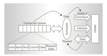
**Figure 16.3:** High-level view of the reinforcement learning DRAM controller. The scheduler is the reinforcement learning agent. Its environment is represented by features of the transaction queue, and its actions are commands to the DRAM system. ©2009 IEEE. Reprinted, with permission, from J. F. Martínez and E. İpek, Dynamic multicore resource management: A machine learning approach, *Micro*, *IEEE*, 29(5), p. 12.
